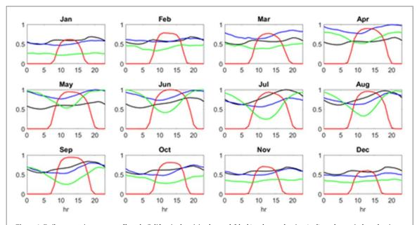
Figure 3. Daily composite averages of hourly California electricity demand (black), solar production (red), onshore wind production (green), and offshore wind production near 46028 (blue) in each month (see text for details). Composite averages are normalized by the maximum over all months and hours of each respective curve. Data from CAISO (http://www.caiso.com/market/Pages/ReportsBulletins/RenewablesReporting.aspx).
