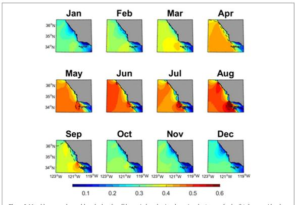
**Figure 5.** Monthly average demand-based values for offshore wind production shown in color (see text for details), for statewide solar production shown as solid contours and statewide land-based wind production shown as dashed contour (contours are typically very close to shore).
