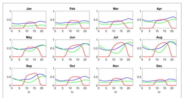
Figure 4. Hourly demand-based values (equation (1)) of solar production (red), onshore wind production (green), and offshore wind production near 46028 (blue) in each month.
