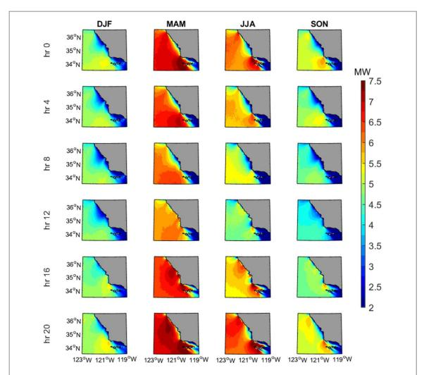
**Figure 1.** Averages of the hourly wind production based on the NREL's 10 MW wind turbine from WIND Toolkit over 2007–2013 at different hours and four seasons. Each column from the left to the right represents winter (December-January-February, DJF), spring (March-April-May, MAM), summer (June-July-August, JJA), and fall (September-October-November, SON). Each row from the top to the bottom represents 00 PST, 04 PST, 08 PST, 12 PST, 16 PST, and 20 PST.
